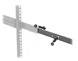
Install the rails onto the chassis by inserting the tabs into the side of the chassis, sliding the rail forward •, and securing the rails with screws •.
