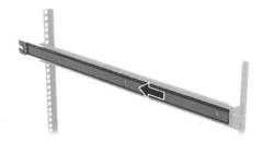
**5** Align the inner rails attached to the chassis with the middle rails, and then insert the chassis into the rack until you feel and hear a click.
