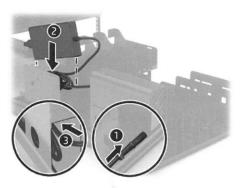
On both inner rails, pull the blue tab forward **1**, and then slide the chassis fully into the rack **2**.
