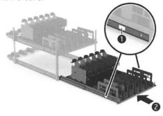
**9** To secure the chassis, tighten the left and right thumb screws on the front of the rack.
